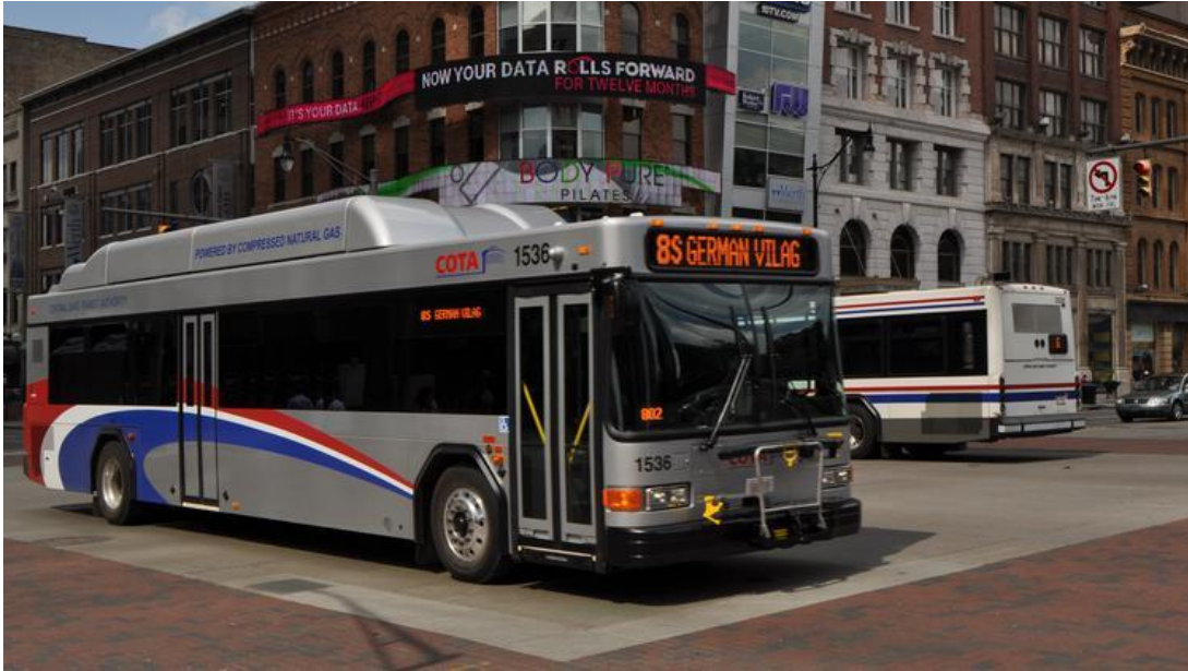
Figure 1: A bus that uses compressed natural gas as its fuel, which produces significantly less emissions.
