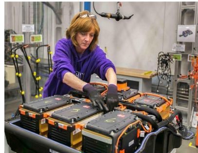
GM Brownstown Battery Assembly Plant Worker Tina Oaks attaches a wiring harness on a Spark EV battery pack Tu May 13, 2014; J.F. Martin for GM, appeared in Detroit Free Press Dec 18, 2018
